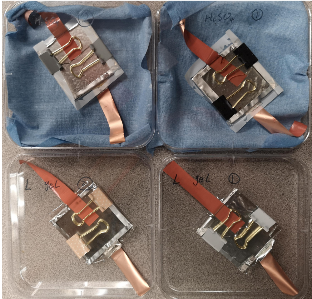
Figure 7: The top two samples were GO/CNTs with an H_2SO_4 electrolyte; the bottom two samples were GO/CNTs with a PVA/ H_3PO_4 gel electrolyte.
